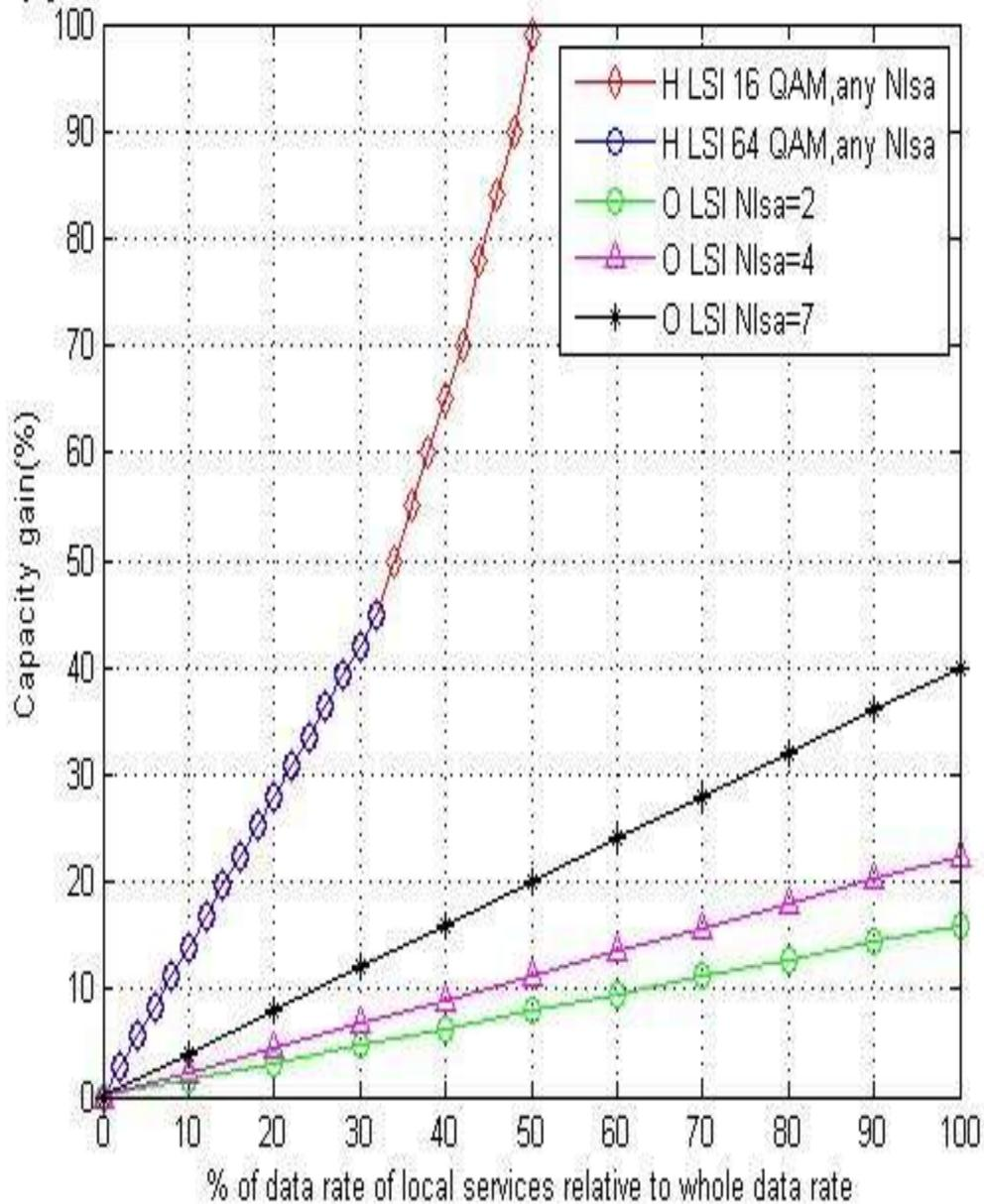
fig 6.6 :- Gain in capacitance of HM-LSI and O-LSI as function of LSAs and the function of local server
