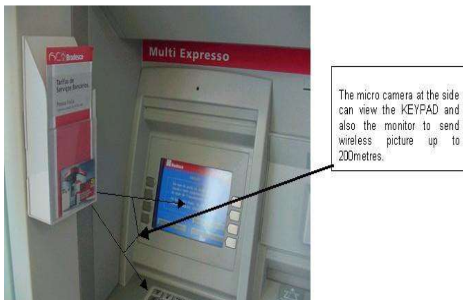
Fig 6. Micro Camera Embedded in Different Positions
