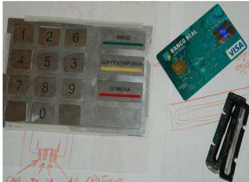
Fig 7. Skimming Device Attached to ATM
