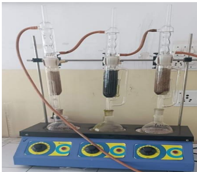
Figure 1: Extraction of leaves, bark and fruits by Soxhlet apparatus
