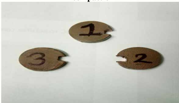
(b) composites sample after the sintering 1) Cu-C 2) Cu - WC 3) Cu-SiC [Source: SGVU, Jaipur]
