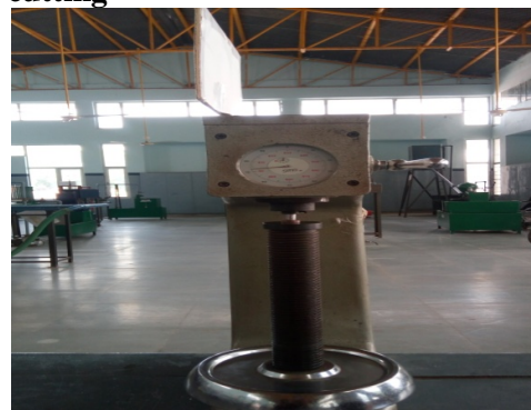
Fig 5. A) Rockwell hardness test b) Hand mill tool used for slot cutting [Source: SGVU, Jaipur], [Source: MSME, Jaipur]
