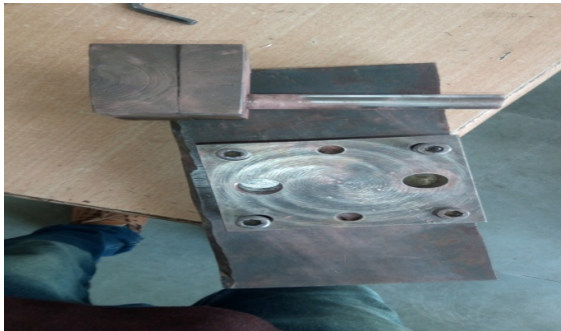
Fig 2. (a) Die (High speed steel) used for compaction
